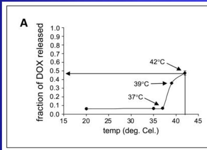
ThermoDox started releasing doxorubicin at a temperature of 39°C. At a temperature of 42°C, release of doxorubicin at 2 min was ~ 50% and nearly 100% by 12 min
